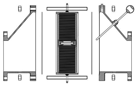
3. On the remaining studs, loosen the holding nuts and use the spreader nuts to separate the base halves from the housing. Use spacer blocks or spreader tools, if necessary, to safely secure the base halves so the housing is free for removal.
