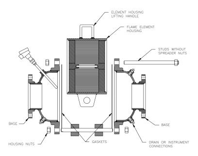
On the remaining studs, loosen the holding nuts and use the spreader nuts to separate the base halves from the
