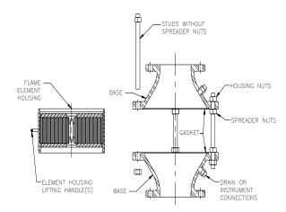
3. On the remaining studs, loosen the holding nuts and use the spreader nuts to separate the base halves from the housing. Use spacer blocks or spreader tools, if necessary, to safely secure the base halves so the housing is free for removal.
