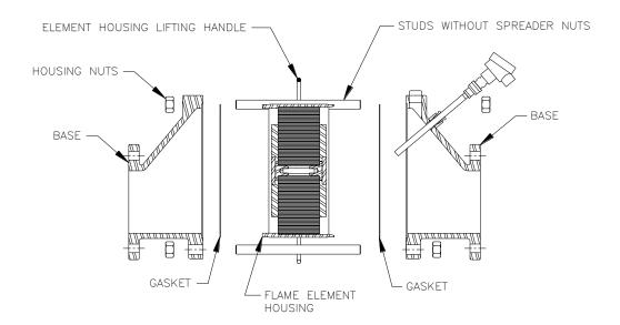
3. On the remaining studs, loosen the holding nuts and use the spreader nuts to separate the base halves from the housing. Use spacer blocks or spreader tools, if necessary, to safely secure the base halves so the housing is free for removal.
