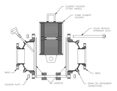
3. On the remaining studs, loosen the holding nuts and use the spreader nuts to separate the base halves from the housing. Use spacer blocks or spreader tools, if necessary, to safely secure the base halves so the housing is free for removal.
